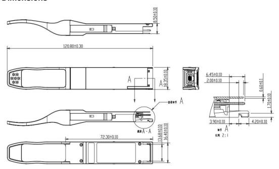
Figure 13. Mechanical Specifications
