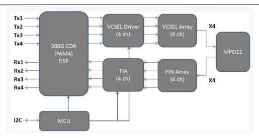
Figure 1. Module Block Diagram
