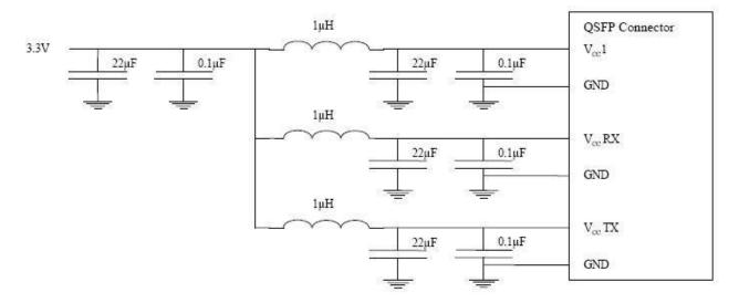
Figure 3. Host Board Power Supply Filtering
