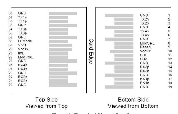
Figure 2. Electrical Pin-out Details
